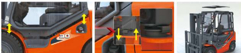
■ suspension cab ■ damping support of the suspension cab ■ panel-mounted cab
